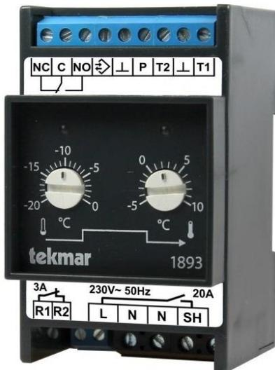
The compact 1893-FGA temperature controller is designed for the use in the areas of de-icing and frost protection. It combines two functions in one device. It can either be used as a dual thermostat with a bottom threshold temperature for the heating function (for example in order to de-ice gutters) or as a self-monitoring control with a bottom alarm temperature (for example for trace heating).
